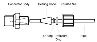
· Push the end of the pipe up to the stop.
